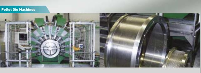
One of our engineers' highlights, unbeatable in precision and productivity. Up to 12 spindles are in use
