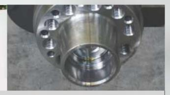
With 1- or 2-fold workpiece clamping, cutting to length, milling, twist drilling, thread cutting in one clamping.
