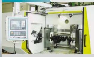
The ENDURO for the end finishing of crankshafts and gear shafts is available in several sizes.
